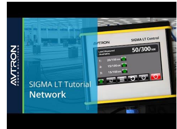
SIGMA LT Tutorials: Load Banks in a Network Learn how to control up to 25 load banks on a network with the SIGMA LT Hand-Held.
